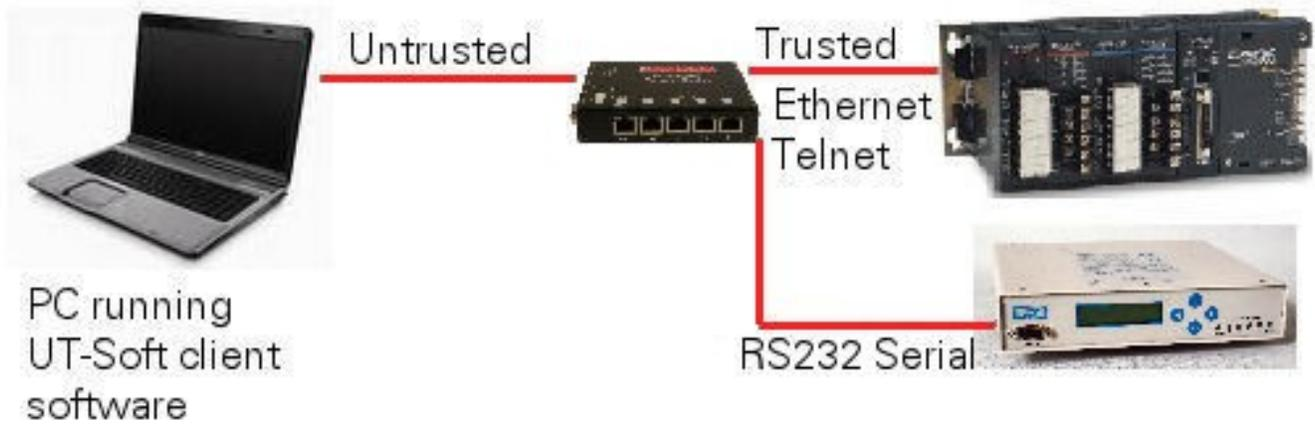
Accessing devices from within a network only requires one UT-3302 server and UT-Soft on the remote work station
