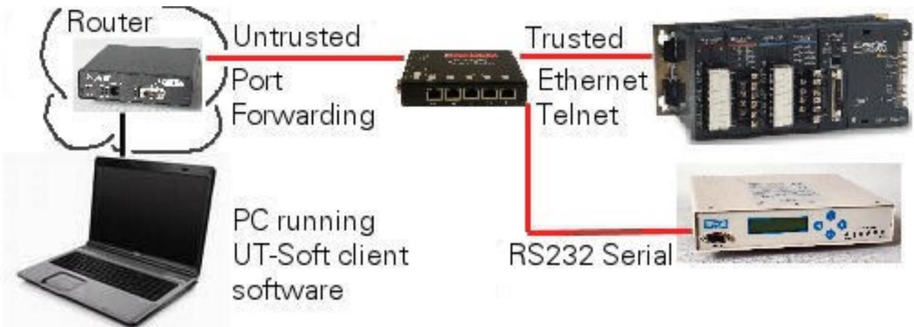
Accessing devices from outside, through the Internet is identical, even if using DHCP or dynamic IP addresses on the remote work stations.
