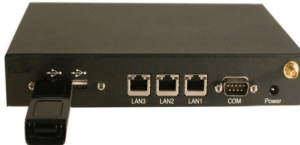
These cellular modems support external antenna options. An adapter cable plugs into the side of the modem. This cable is then connected to an antenna. External antennas are used when the modem is in a metal enclosure, when the distance from the cell site to the ET-6601 calls for an external antenna or an amplifier, and similar situations where the modem's internal antenna is not sufficient to receive a good signal.
