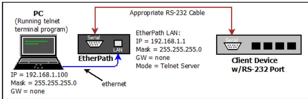
Figure 1 – Configuration for Telnet Server Mode, with Example IP Address on EtherPath
