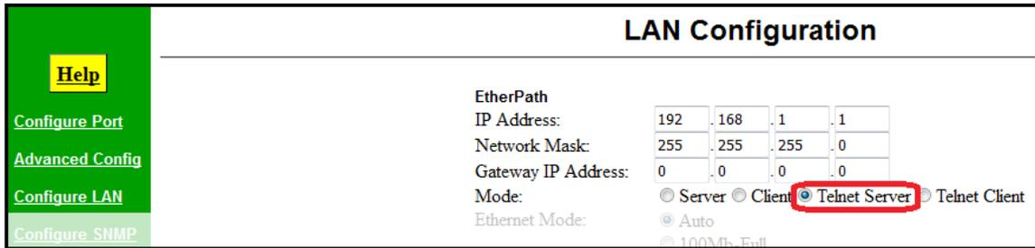
Figure 3 – Selecting Telnet Server on Configure LAN Screen
